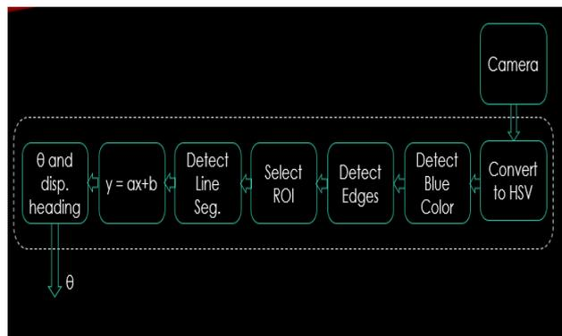
Figure7. The Lane Detection Process
